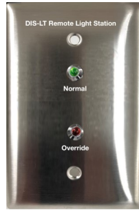
Example of a RILS with smaller labelling and less words on an industry standard cover plate..
